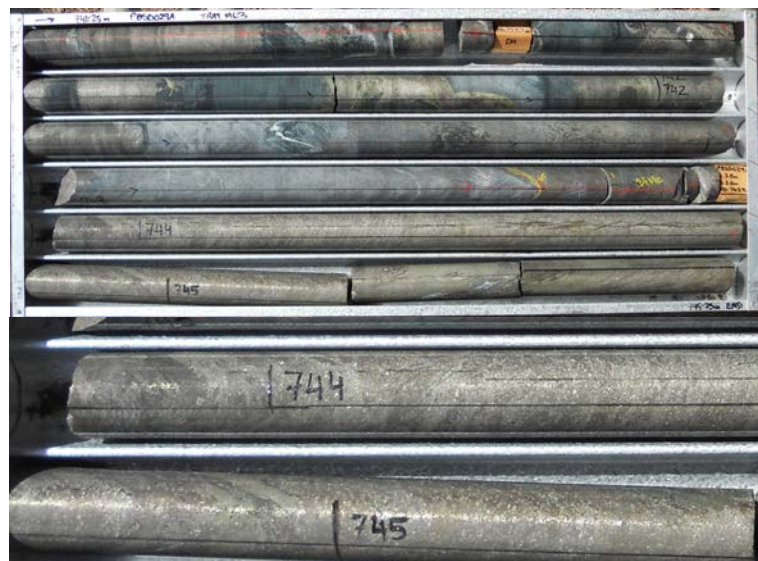
Figure 1: Mineralised drill core from PBS0029A showing the channel base at the start of the core tray with incorporated felsic clasts and then massive sulphide formation
