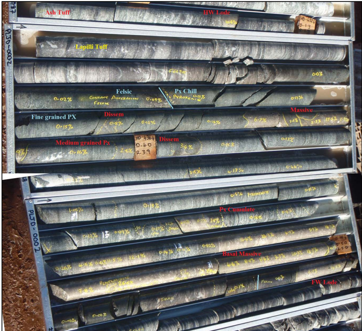
Figure 3: Complete intersection of massive, stringer and disseminated nickel sulphides within pyroxenite ultramafic in PLJD0002 (432.0m-443.0m)
