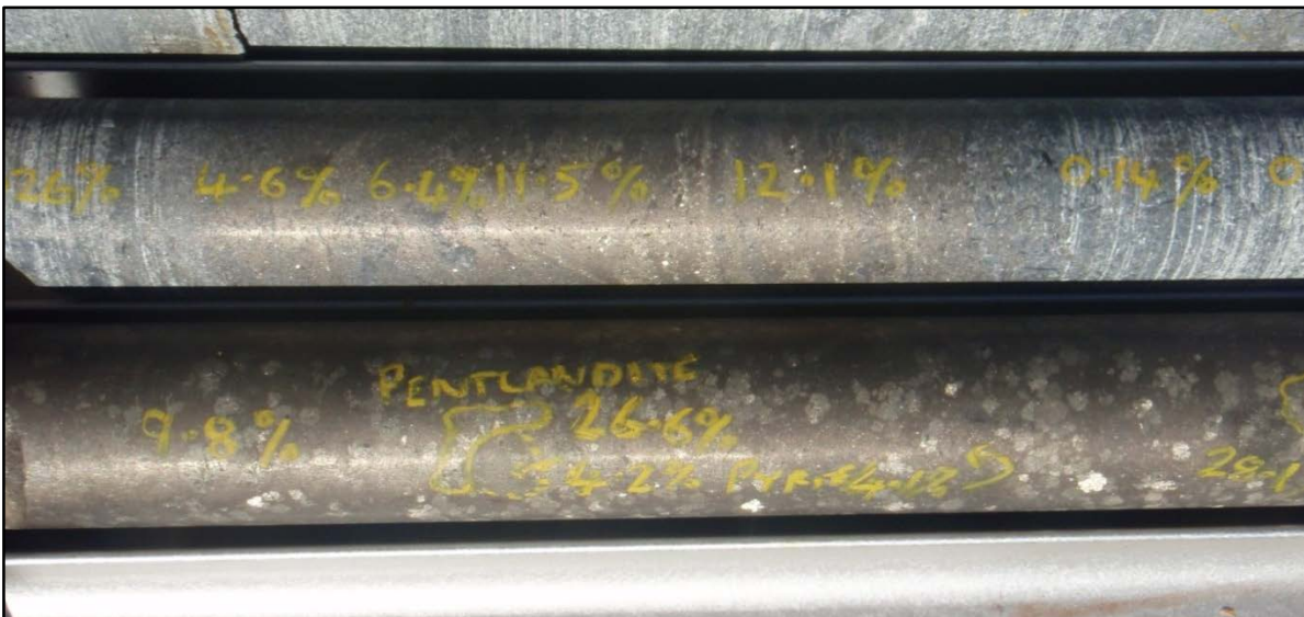
Figure 2: High grade massive nickel sulphide (pentlandite) intersected in PLJD0002 (439.6-440.8m depth) 350m north of Emily Ann mine
